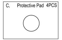
• Attach the protective pad (C) under the adjusting knob.
